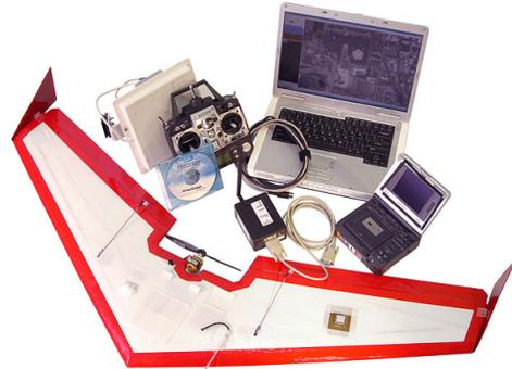
Figure 1: Unicorn Unmanned Aerial System from Procerus.
