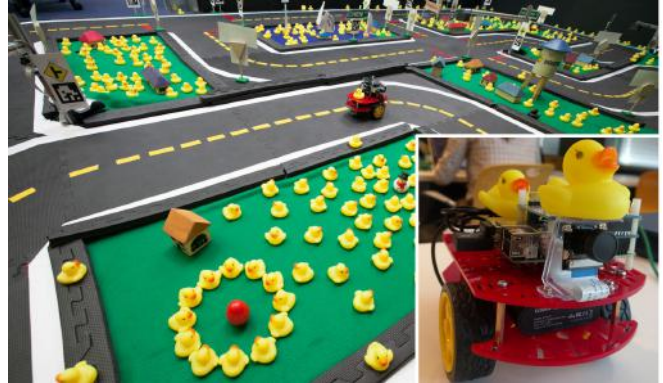
Fig. 1. In Duckietown, inhabitants (duckies) are transported via an autonomous mobility service (Duckiebots). Duckietown is designed to be inexpensive and modular, yet still enable many of the research and educational opportunities of a full-scale self-driving car platform.
