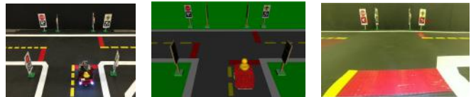
Fig. 12. Global localization. Left: The real Duckiebot at an intersection in Duckietown, Middle: The Duckiebot having localized within the map, Right: The internal camera view with the sign detections highlighted.
