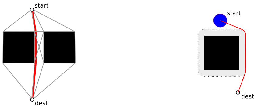
(a) Computing the shortest path using the visibility graph. The task is to find the shortest path from start to dest such that the obstacles, depicted in black in the picture, are avoided. The visibility graph is shown in gray, the shortest path on the graph is highlighted in red.
